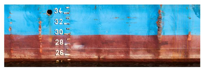
The heavier a vessel becomes, the higher draft that is required. Under normal conditions, the Panama Canal can accommodate a draft of up to 50 feet. Under current conditions, draft restrictions are set at 44 feet. The net impact for vessels that were specifically designed to maximize the beam (width) and draft (depth) restrictions of the canal is they can only be loaded to 80-85% capacity.
